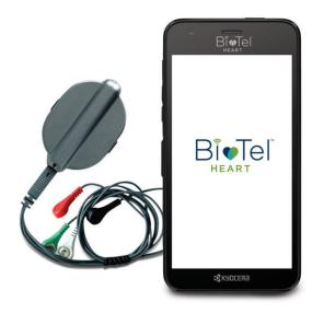
The device is comprised of two (2) main components: 1) a patient-worn sensor with 3 leads and 4 electrodes and 2) a monitor. The device continuously monitors patient ECG, automatically generates an alert triggered by a proprietary detection algorithm, or generates an alert manually triggered by the patient, and transmits the recorded data transtelephonically via Bluetooth to a monitoring center 24 hours a day.
