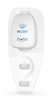
The device is comprised of two main components: 1) a patient-worn sensor with no leads and two channels and 2) a monitor.
